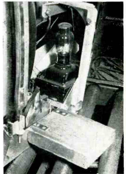
Angle brackets hook over side of chassis to hold spacer block
