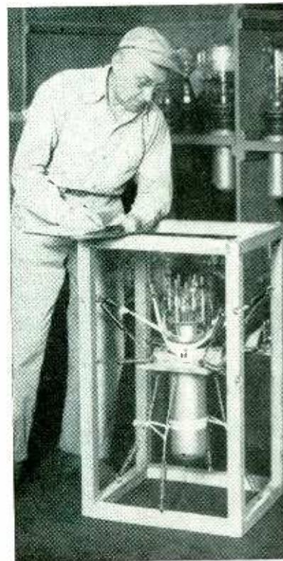
Sixteen stiff coil springs support and position this heavy transmitting triode within its wood shipping frame
