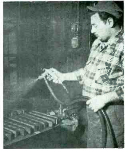
Spraying masked i-f transformers for tropicalization. Two-shelf conveyor in background carries other sprayed units into baking oven near ceiling
