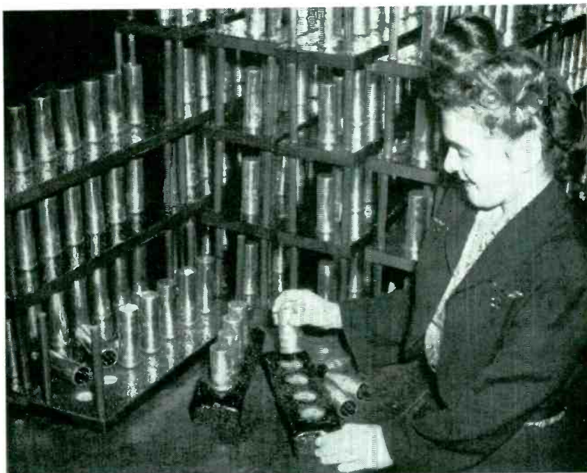
Re-usable terminal masks for plug-in electrolytics. Those in background have wood-dowel corner posts to permit stacking for air drying after spraying
