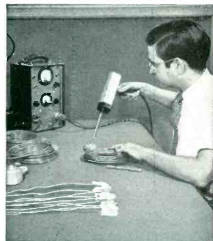
SENSITIVE EQUIPMENT, such as this Type H Leak Detector, functions accurately only when voltage is properly stabilized. G-E voltage stabilizers perform this stabilizing function.
