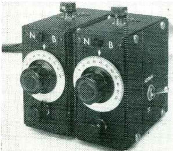
Two units containing elements shown in Fig. 3 may be used together to provide an extremely flexible arrangement with a choice of two nulls, two peaks, or one of each for separating desired and interfering signals
